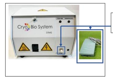
⇒ Pressing the white "\$1" pushbutton or the "U2" control pedal (available as an option) activates a welding cycle.
