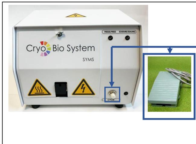
⇒ Pressing the white "S1" pushbutton or the "U2" control pedal (available as an option) activates a welding cycle.
