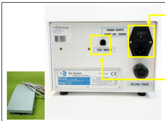
⇒ Connect the mains power cable "Cb1" to the socket in the input filter "U0" identified by: **POWER SUPPLY**
