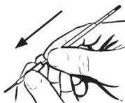
1. Insert straight and firmly the side of the CBS™ High Security straw that is to contain the biological sample into the filling nozzle. A click can be perceived. The central capillary enters the straw without touching the inner surface. Check the connection by applying slight withdrawal force on the filling nozzle that should not move.
